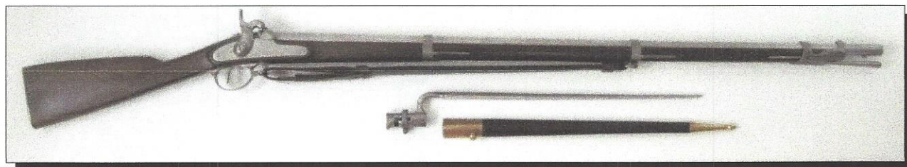
M1842 .69 cal. smoothbore musket with socket bayonet and M1828 scabbard.
